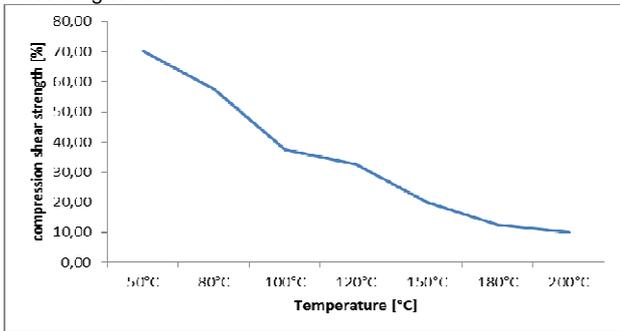
tensile strength after temperature storage
