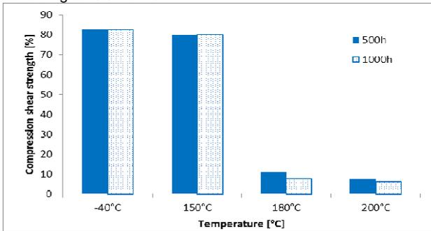
compression/shear strength shaft-hub joint at temperature
