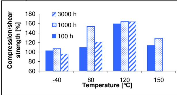
compression/shear strength glass/glass at temperature
