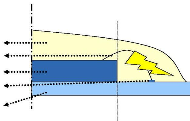
Because the majority of these adhesives are used to protect bare semiconductors, it is important that any outgassing from the adhesive is kept to a bare minimum. All the encapsulation products in the Inseto range of materials meet this requirement, with measured ionic impurity levels of <10ppm.
