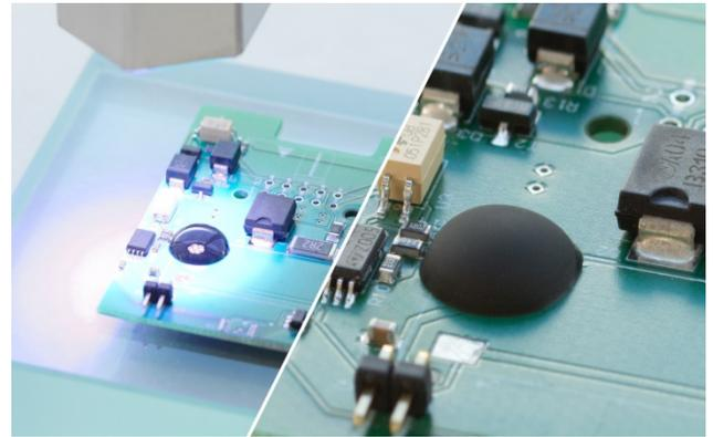
The curing process is a combination of the two already outlined: UV flash on the surface for 5 seconds at 200mW/cm<sup>2</sup>, and then oven cure at 150C for 30 minutes. Comparisons against the existing GE725 Fill show no degradation in chemical resistance:
