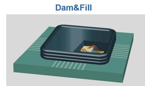
As a general rule-of-thumb, Globtop is used for areas up to 2mm x 2mm, and then Dam & Fill takes over.
