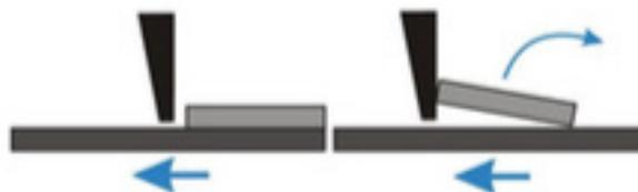
Die shear testing may involve the application of very high shear loads and can currently be tested up to 200KG!
