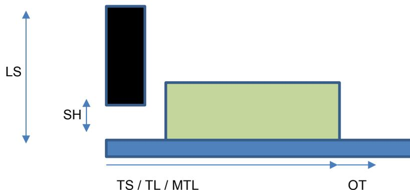
Diagram 1 – shows the point at which different parameters take place during shear testing.
