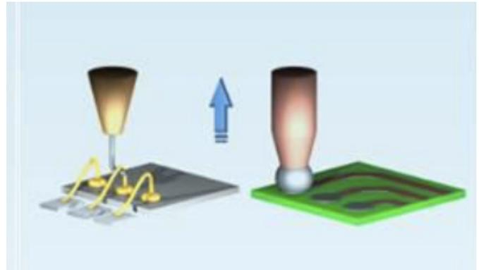
**PUSH-PULL** is used to test solder joints, where the joint or component is loaded first one way and then the other. The tool applies the set load first in one direction and then in the opposing direction, repeating this cycle. The displacement is adjusted automatically to get the desired load.
