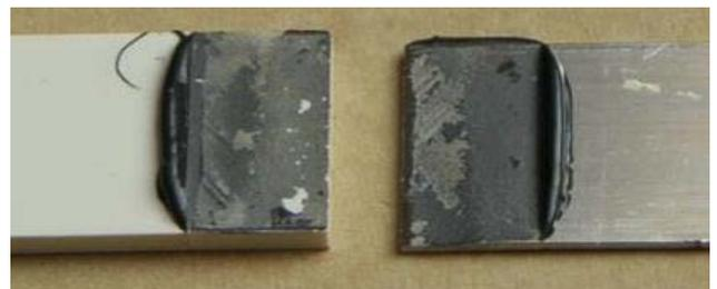
Flexibility – there are different ways to indicate the flexibility of an adhesive: elongation, Young’s Modulus, sometimes shore hardness. Elongation is the easiest to both measure and visualise – it is calculated in the same test that determine the tensile strength of the adhesive. The percentage that the test coupon has strength when it breaks is the elongation, also specified in the data sheet – simple!
