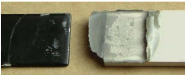
Adhesive bond strength is defined as the bond strength of the adhesive to the materials being bonded. **In every case**, this has to be tested in the specific application under discussion. No two materials give the same bond strength, so an adhesive that bonds well to stainless steel might be terrible with aluminium. Even within a generic material such as Polycarbonate, care needs to be taken.
