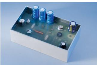
**Casting.** This is typically for circuitry intended for use in harsh environments; to protect the PCB from moisture and contamination (see photo). The adhesive-of-choice would be a two-part epoxy, as they are relatively low cost and a significant volume might be required for some applications. Pre-use storage and curing (which takes about 24 hours) is at room temperature.
