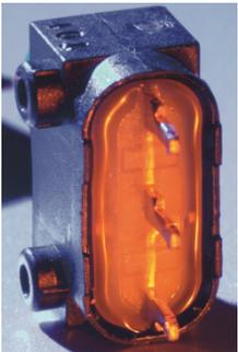
**Socket securing and pin coating/sealing.** This is done mainly to prevent moisture ingress and to reduce the risk of dendritic growth. There are two options available for securing/bonding pins/sockets. The first is to use a light-cured epoxy (see photo). These are popular as they cure very quickly in the presence of a high intensity light-source, making them ideal for high volume, rapid-turnaround production runs.
