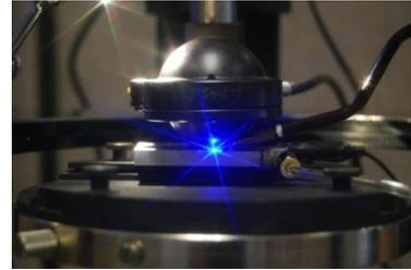
For all sphere configurations, the sphere must be held securely in place a short distance from the emitter. The integrating sphere must be held just above the device under test (DUT) leaving just enough room for contacting probes.
