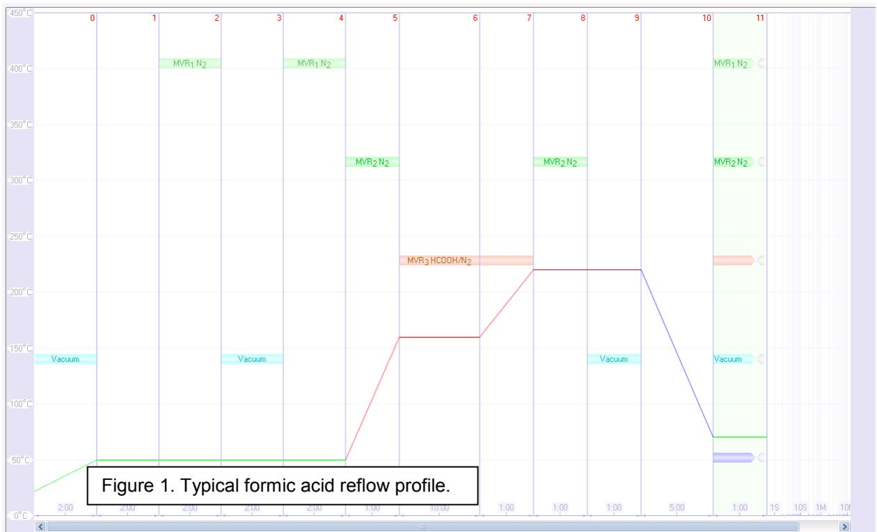
Figure 1. Typical formic acid reflow profile.
