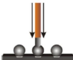
10. Once the final temperature has been reached (T6 in the temperature profile) the test pin is clamped and the pull test automatically carried out.
