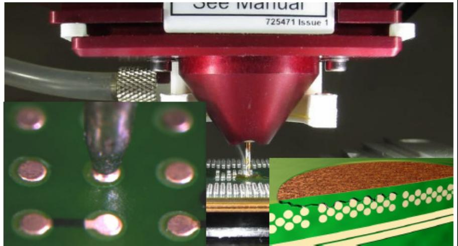
HBP testing is applicable to both traditional solder ball and flip chip bumps either bonded or formed by the deposition process and is also used to identify pad crater failures on the substrate side (IPC 9708). Generally, HBP testing is destructive. However, you can configure the test to be non-destructive if required.
