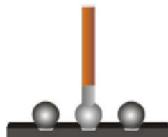
9. During the cooling phase of the temperature profile, air is directed down onto the test site (see note below)
