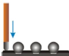
6. If required, raise the Z axis and carefully apply a small amount of flux to the test pin-tip. Position the test pin over the ball/bump to be tested. Ensure it is aligned correctly in both X and Y axes.
