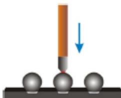
8. Start the test. The temperature is controlled by the current temperature profile and its status reported in the Paragon software. The solder melts and re-flows and the test pin drops into the ball/bump.
