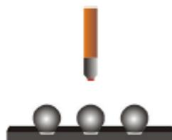
7. Lower the Z axis until the test pin-tip just touches the ball and inspect alignment. Lower Z axis to the preset Lower Limit.
