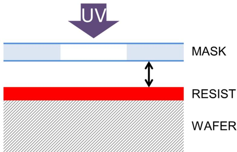
Typical exposure of wafer and mask within a mask aligner.
