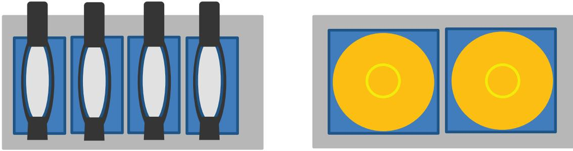
Wedge Bond versus Ball Bond Pitch Comparison
