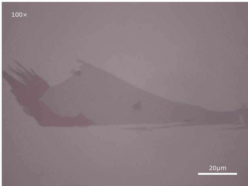
Single and bi-layer graphene flakes on 90nm of thermally grown SiO<sub>2</sub>, (image courtesy of Graphene Industries Ltd)
