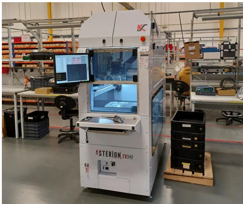
Above, the Asterion EV wedge bonder in situ within Steatite’s Power Business Unit.
